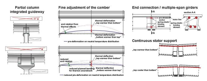
Fig. 8 Proposed modifications to the structural systems for temperature effect amendment
