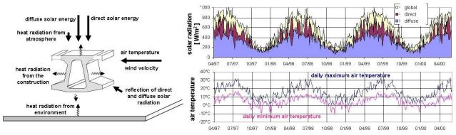
Fig. 2 Thermal environment of guideways on the testing facility in Emsland/Germany
