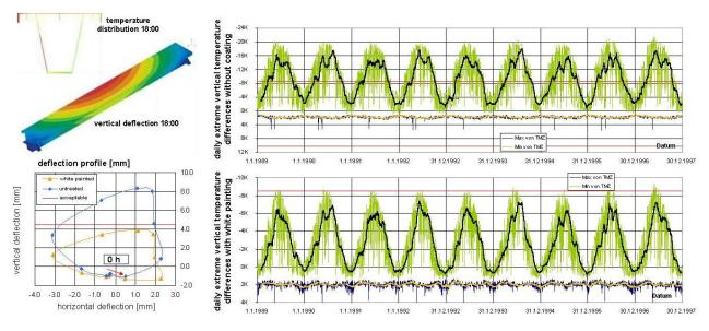
Fig. 5 Results of analysis for a single-span steel girder
