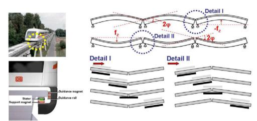
Fig. 1 Levitation system of Transrapid, Kinks caused by guideway deflections
