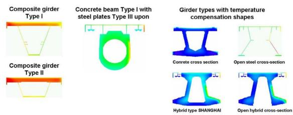
Fig. 7 Temperature distributions over alternative cross-sections
